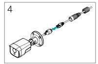
4 Connect the plug terminal to the RJ45 jack.
